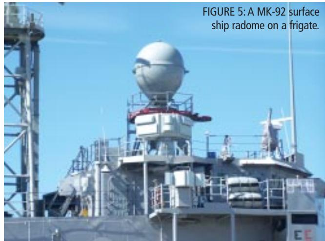
FIGURE 5: A MK-92 surface ship radome on a frigate.
