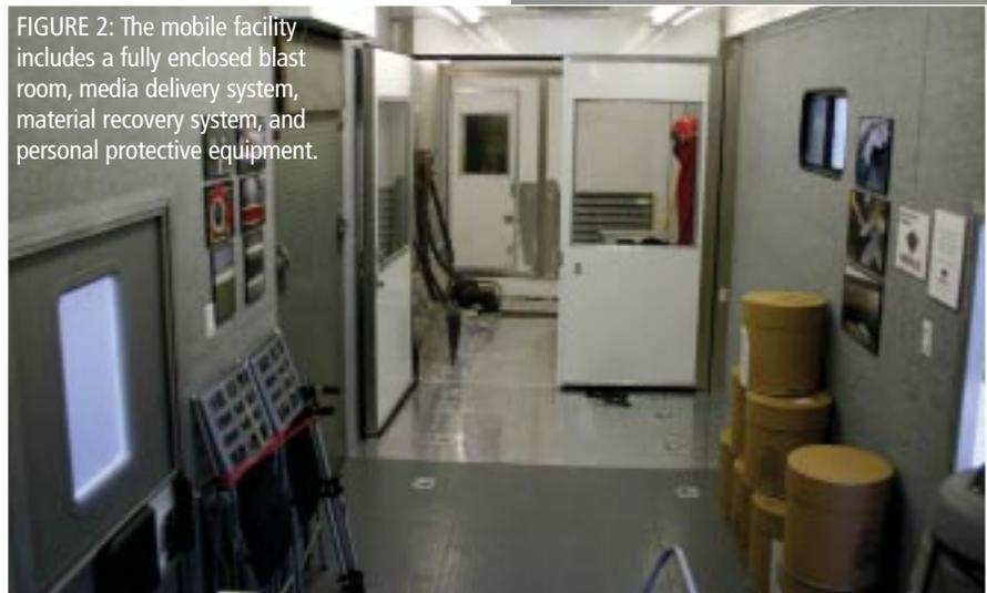
FIGURE 2: The mobile facility includes a fully enclosed blast room, media delivery system, material recovery system, and personal protective equipment.
