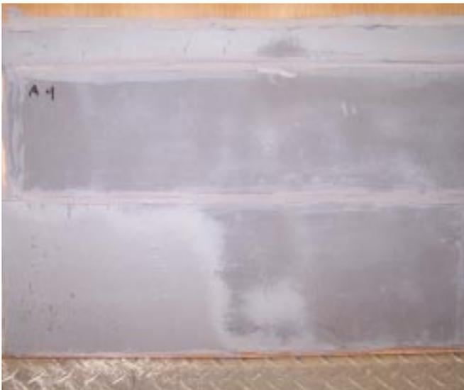
FIGURE 8: Coatings were removed from the PCMS radar-absorbing material at a rate of 35 ft<sup>2</sup>/hr with no visual damage.
