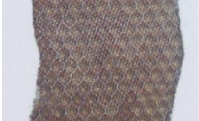
FIGURE 4: Coatings were removed from the P-3 Orion aircraft radome panel at a rate of 12 ft<sup>2</sup>/hr with no visual damage.
