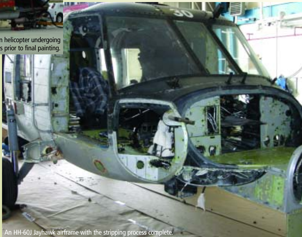
While some minor chemical stripping is required in some sensitive areas, the majority of the stripping is accomplished using the cornstarch media.
