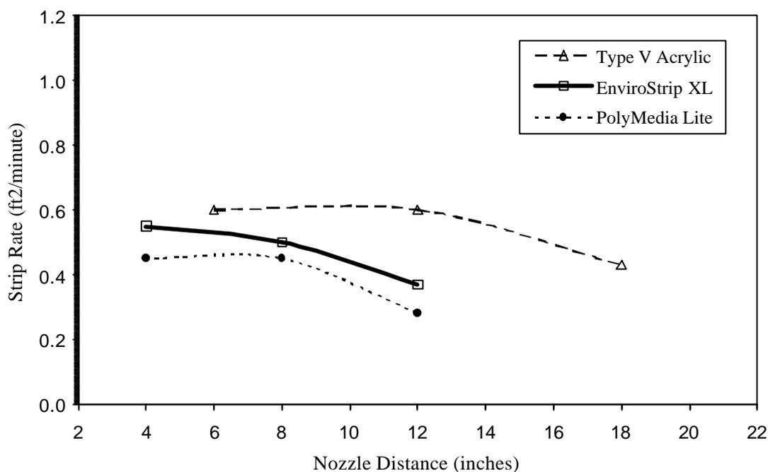
**Figure 6.** Plot of Strip Rate versus Nozzle Distance on Panel Type “C” for Type V Acrylic, ENVIROStrip<sup>®</sup> XL, and PolyMedia Lite 75
