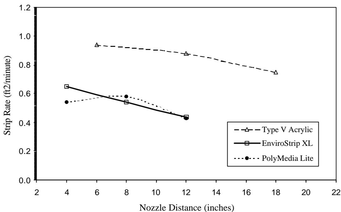
**Figure 4.** Plot of Strip Rate versus Nozzle Distance on Panel Type “A” for Type V Acrylic, ENVIROStrip<sup>®</sup> XL, and PolyMedia Lite 75
