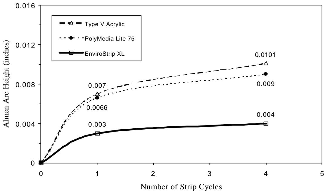
**Figure 3.** Plot of Almen Arc Height versus Strip Cycle for Type V Acrylic (18-inch distance), ENVIROStrip<sup>®</sup> XL and PolyMedia Lite 75 (12-inch distance)
