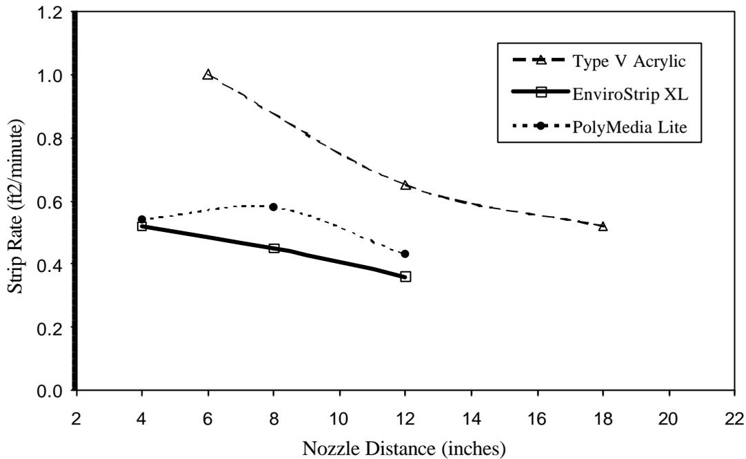
**Figure 5.** Plot of Strip Rate versus Nozzle Distance on Panel Type “B” for Type V Acrylic, ENVIROStrip<sup>®</sup> XL, and PolyMedia Lite 75
