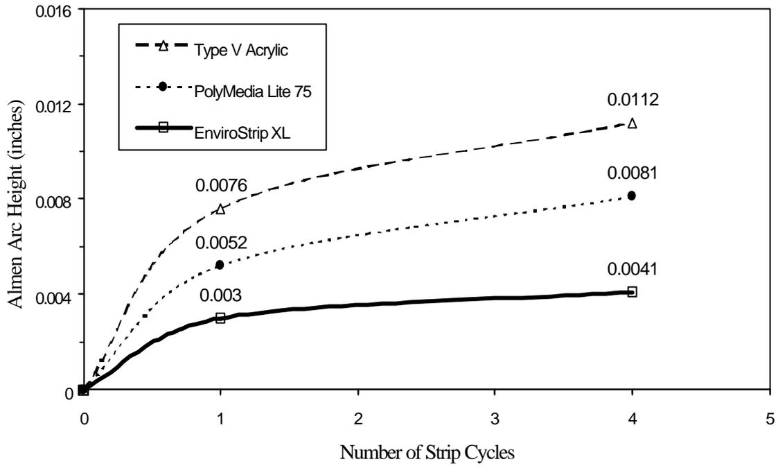
**Figure 2.** Plot of Almen Arc Height versus Strip Cycle for Type V Acrylic (12-inch distance), ENVIROStrip<sup>®</sup> XL and PolyMedia Lite 75 (8-inch distance)
