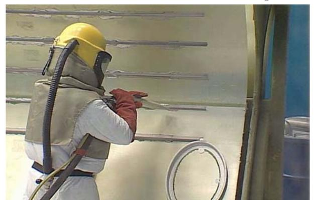
**ABOVE: Operator applying the Envirostrip process to a large metal bonded structural part.**
