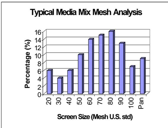
Figure C-1 Mesh Size of Typical Production Mix
